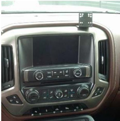
InDash installed showing Right mounting location
