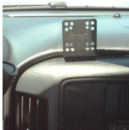
InDash installed showing Left mounting location
