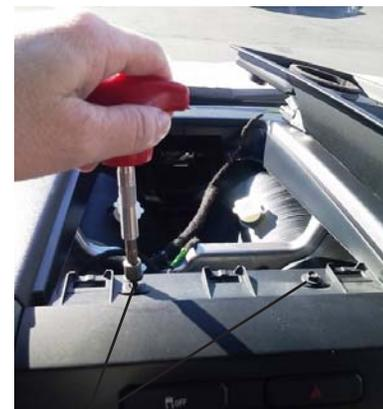
Screws to remove radio bezel
